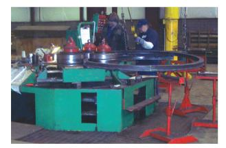
Olson's 300-ton hydraulic bulldozer allows us to form beams and channels up to 24-inches deep. The machine can also be used to straighten structural tees after splitting or to straighten materials that have been distorted due to extensive welding or galvanizing.
